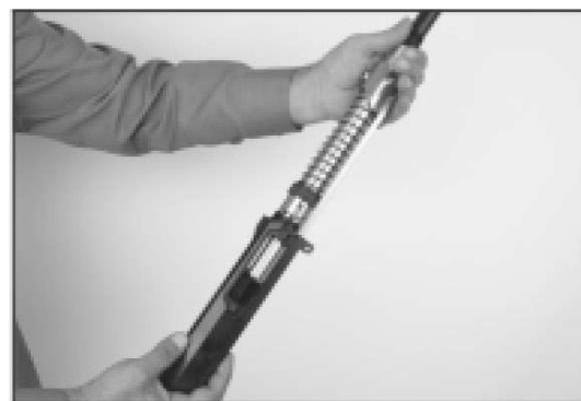
11) Separate the Barrel from the Upper Receiver
